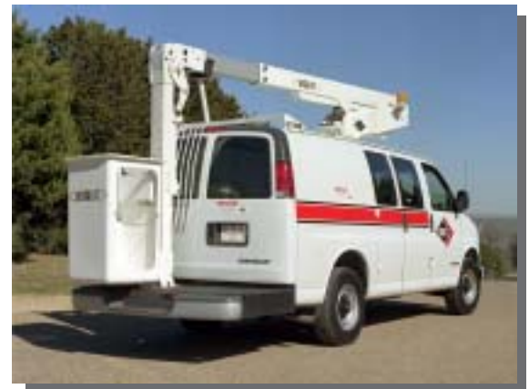
The flyboom gives easy access to the platform from the tailshelf.
