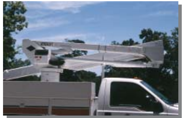
Side by side low stow boom design allows for safer platform entry and reduced travel height.
