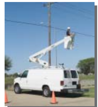
Remote controls allow operation from the ground.
