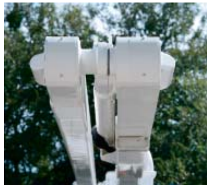
Boom Knuckle Protects Cylinder.
