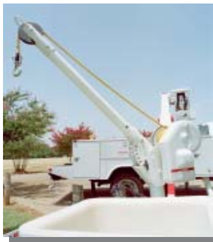
Jib & winch provide 800 lbs of material handling capacity.
