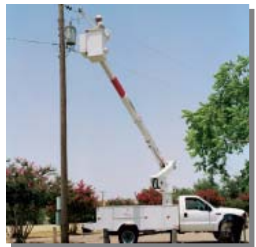
The working height is over 40 feet, with standard pedestal.
