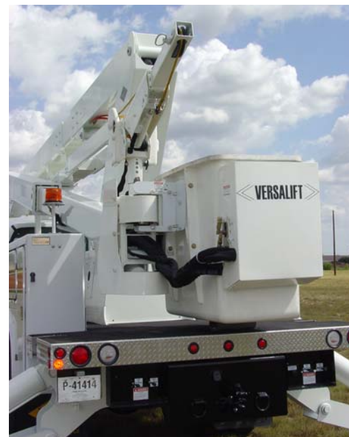
Optional Material Handling Jib & Winch provides up to 2,000 lbs. of material handling capacity.
